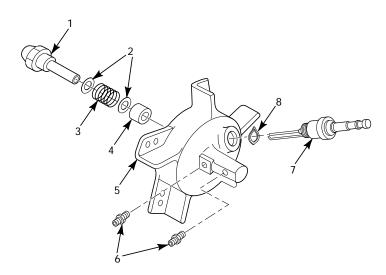
Figure 22 - Burner Head Assembly
